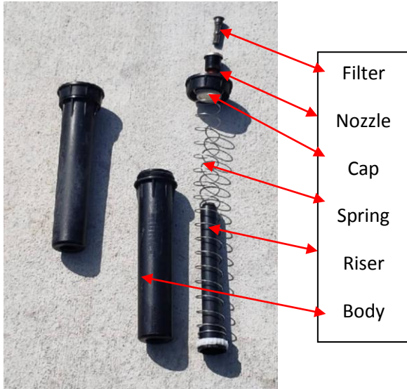
The sprinkler on the left is in most yards. On the right is the same type disassembled.
